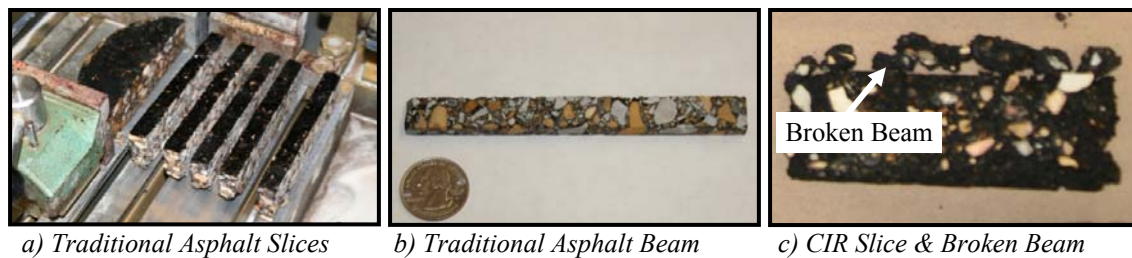
Figure 3.1 Example BBR Specimen Preparation for Traditional Asphalt and CIR
