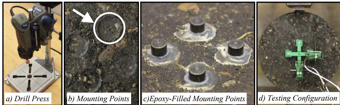
Figure 7.2 Instrumented Specimen Preparation
